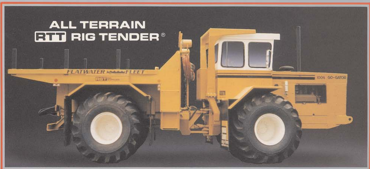
RTT-RIG TENDER with 1,000 gal. (3,800 L) water and 300 gal. (1,140 L) fuel mounted on an all-terrain, articulated, all-wheel drive carrier. Tenders are also mounted on tracked all-terrain carriers.
