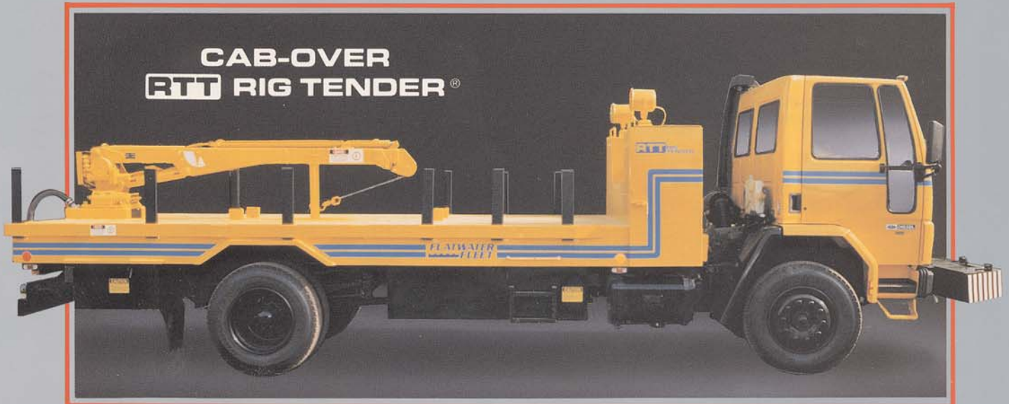
RTT-RIG TENDER with 1,000 gal. (3,800 L) water and 150 gal. (570 L) fuel mounted on a cab-over single axle diesel truck.
