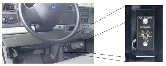
An in-cab control console for accessory components, centralized for added convienience and protection against fuel theft.
