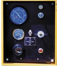
Centralized control panel for engine, high pressure pump, and FRAC-PACKER $^{TM}$ .
