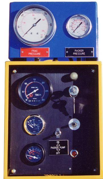
Centralized control panel for engine, high pressure pump, and FRAC-PACKER<sup>TM</sup>.
